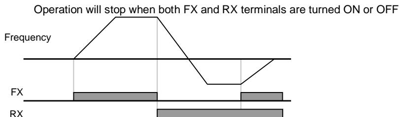
Run command setting 2 at FX and RX terminals
